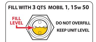
To read correctly, get eye level with sight glass while unit is sitting level, and check that oil level is even with the head of the red arrow. Add or drain oil accordingly.
